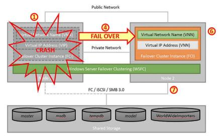
FIGURE 4-37 Failover Clustering Fail Over
