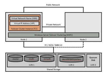
FIGURE 4-36 Failover clustering architecture
