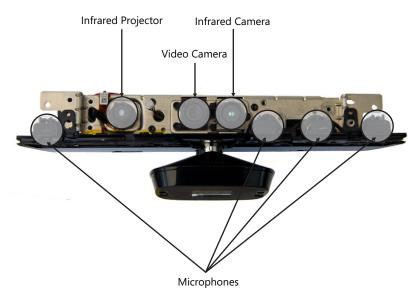
FIGURE 1-2 A Kinect sensor unwrapped.
