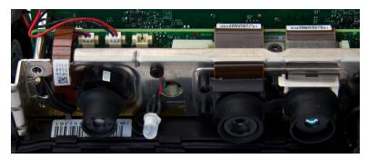
Figure 1-4 shows the arrangement of the infrared projector and sensor.
