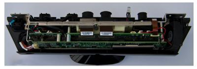
FIGURE 1-3 The Kinect sensor data processing hardware.
