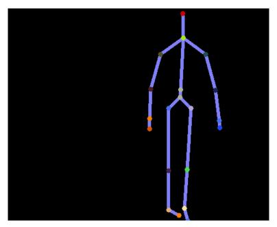
FIGURE 1-9 Skeleton information retrieved using the Kinect software.
