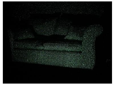
In contrast, Figure 1-6 shows how the Kinect infrared sensor sees the same view.
