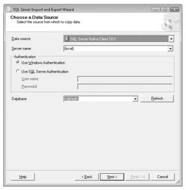
**FIGURE 1-3** The Import And Export Wizard first lets you choose the data source where the data will be coming from, such as a SQL Server database, an Excel spreadsheet, or a flat file.
