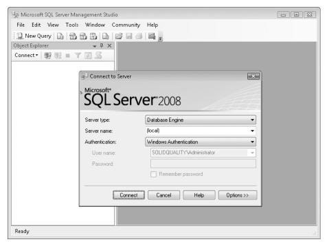
**FIGURE 1-1** Start SSMS by selecting Microsoft SQL Server 2008 from the Start menu and then selecting SQL Server Management Studio. Connect to the Database Engine to manage SQL Server relational databases.
