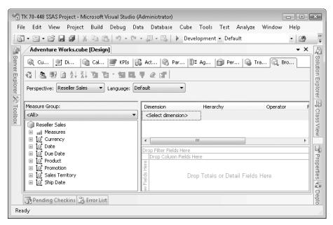
FIGURE 6-13 The Reseller Sales perspective filters the cube metadata to show only the cube objects that are included in the perspective.
