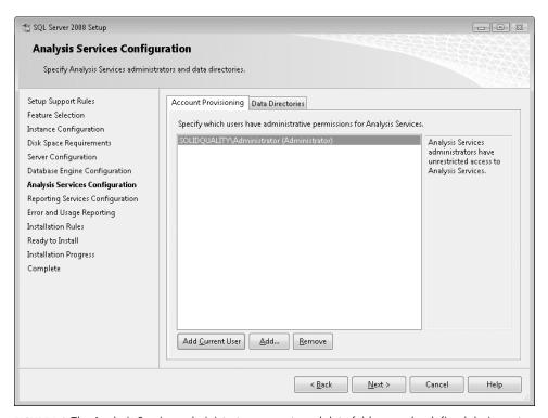
FIGURE 1-6 The Analysis Services administrator accounts and data folders can be defined during setup.
