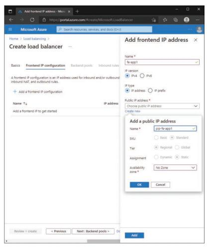
FIGURE 3-11 Load balancer frontend IP configuration
