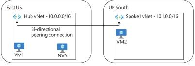
FIGURE 3-5 NVA proxy diagram
