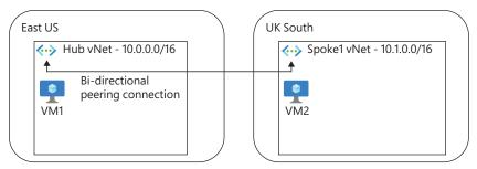
FIGURE 3-1 Bi-directional communication with virtual network peering
