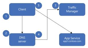
FIGURE 3-46 Traffic Manager DNS diagram
