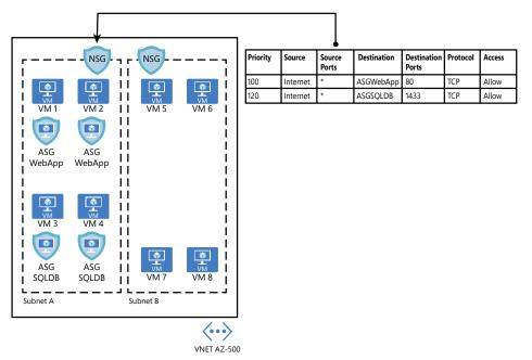
FIGURE 2-18 ASG used as the destination in the NSG routing table
