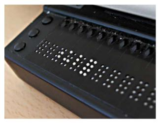
FIGURE 5-1 The refreshable Braille display
