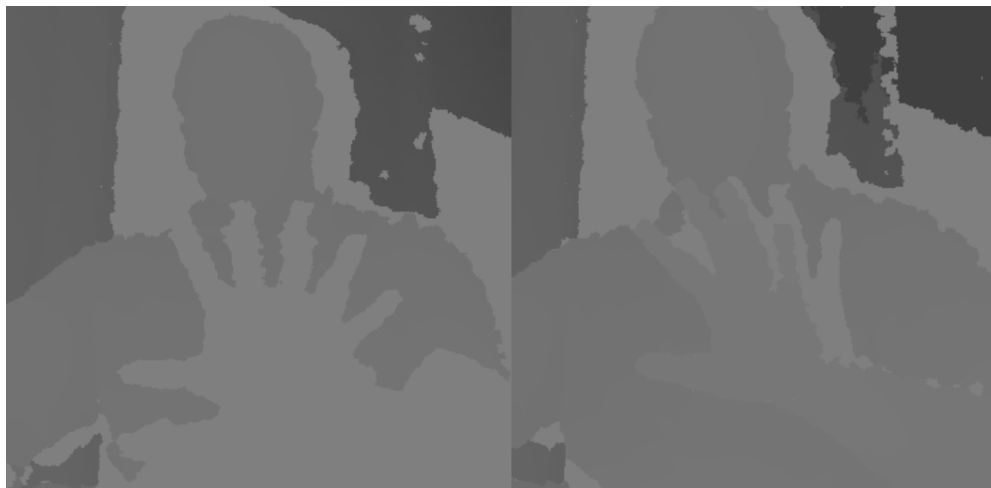
FIGURE 3-4 Hand depth values out of range in standard mode are shown at left, and hand depth values in range in near mode are shown at right.
