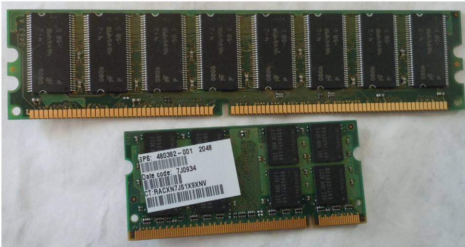
FIGURE 3-2 Comparing a DIMM and a SODIMM.
