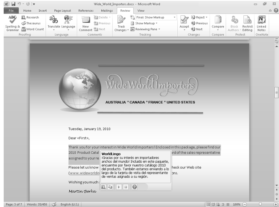
Figure 1-4 The Mini Translator pops up over your Word window and enables you to copy, look up, or listen to the translation.
