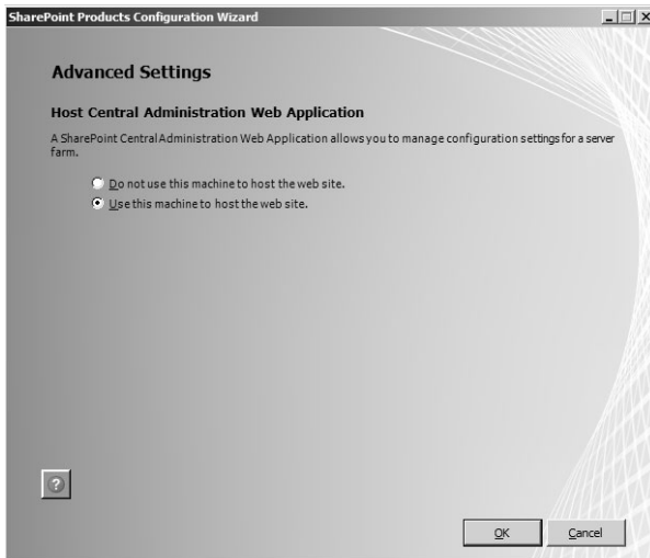
FIGURE 3-4 Select Use This Machine To Host The Web Site, and click OK.
