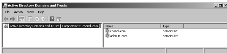
FIGURE 7-4 Use Active Directory Domains And Trusts to work with domains, domain trees, and domain forests.
