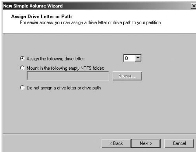
FIGURE 12-4 On the Assign Drive Letter Or Path page, assign the drive designator or choose to wait until later.
