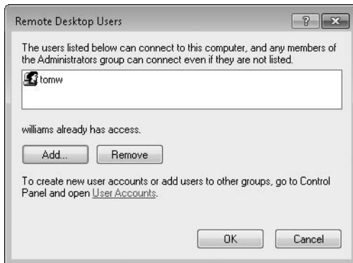
FIGURE 5-15 Specify the additional users allowed to make Remote Desktop connections.
