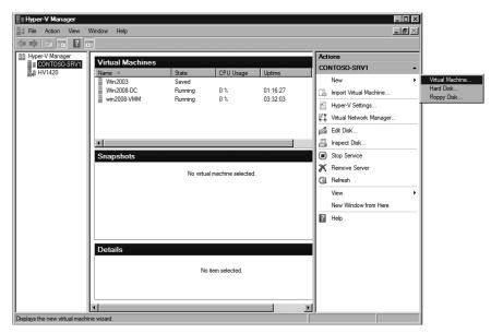
FIGURE 2-5 Creating a new virtual machine in Hyper-V Manager
