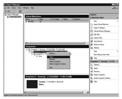
FIGURE 2-13 The Snapshot Apply option in the Hyper-V Manager console
