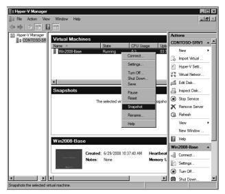
FIGURE 2-9 Creating a virtual machine snapshot using the Hyper-V Manager console
