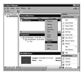
FIGURE 2-12 The Snapshot Revert Option in the Hyper-V Manager console
