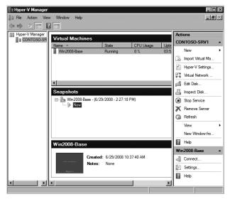
FIGURE 2-10 Snapshot display in the Hyper-V Manager console
